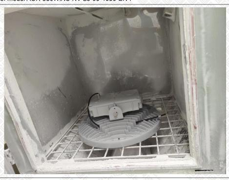
Photo 4: IPX6 test of model AOK-580WiNS-NV-L5-00-4080-BN-P
