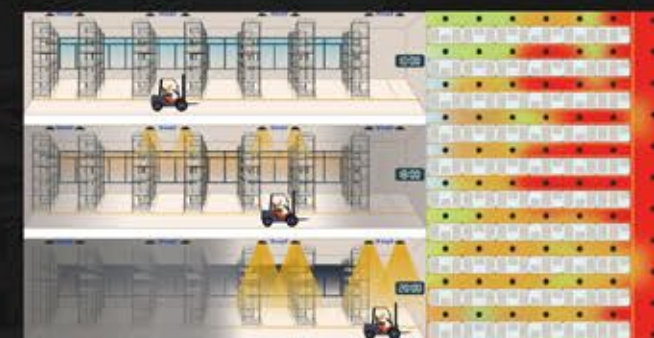
Motion (2-step dimming) + Daylight Sensor (constant illuminance)
