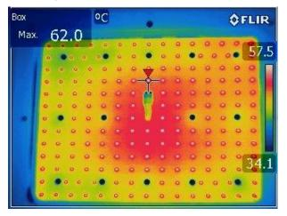
Temperature measurement point on TMP<sub>LED</sub>(at 50°C)
