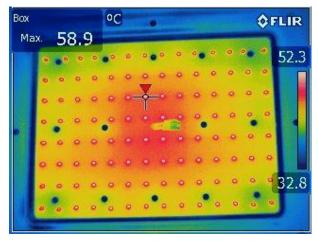
Temperature measurement point on TMP<sub>LED</sub>(at 50°C)
