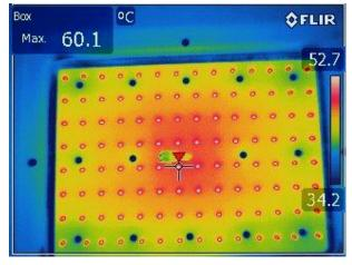
Temperature measurement point on TMP<sub>LED</sub>(at 50°C)
