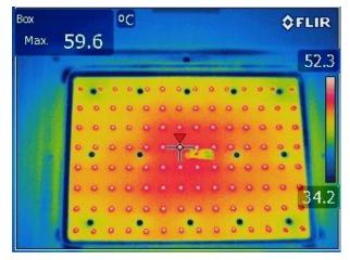
Temperature measurement point on TMP<sub>LED</sub>(at 50°C)
